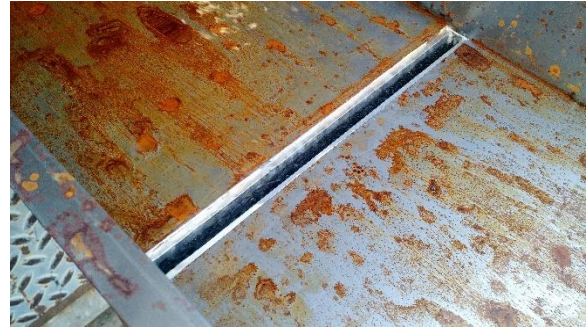
Figure 10: Drain at 1/40 grade, 6 GPM
