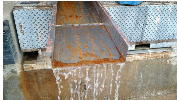
Figure 12: Flow at 1/40 grade, 11 GPM
