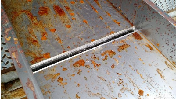
Figure 7: Drain at 1/8 grade, 5 GPM
