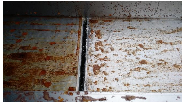
Figure 11: Drain at 1/40 grade, 11 GPM
