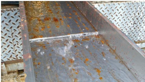
Figure 8: Drain at 1/8 grade, 9.5 GPM
